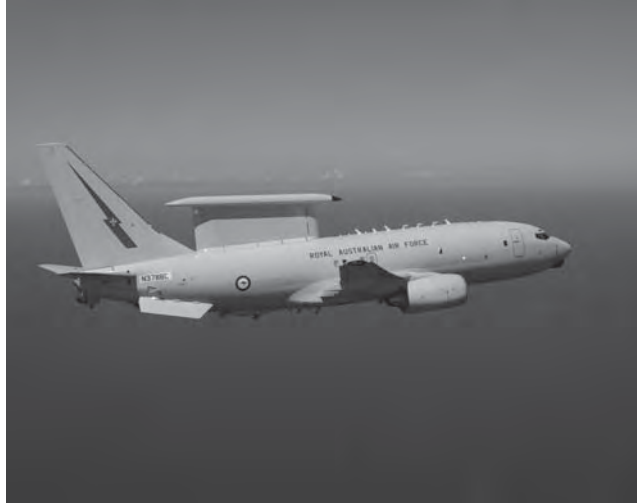
FIGURE 3.2 Boeing 737-700 Wedgetail aircraft showing antennas mounted above the fuselage
