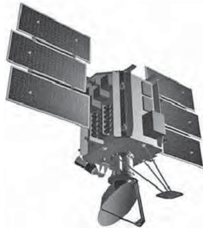
FIGURE 18.19 The Seawinds scatterometer, as embarked on Japan's ADEOS-II spacecraft. The radar drives the conically scanned reflector antenna, which takes up most of the real estate on the Earth-viewing face of the satellite.
