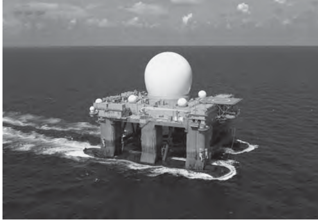
FIGURE 13.50 SBX—over 250 ft tall and displacing more than 50,000 tons (Courtesy of Raytheon Company)
