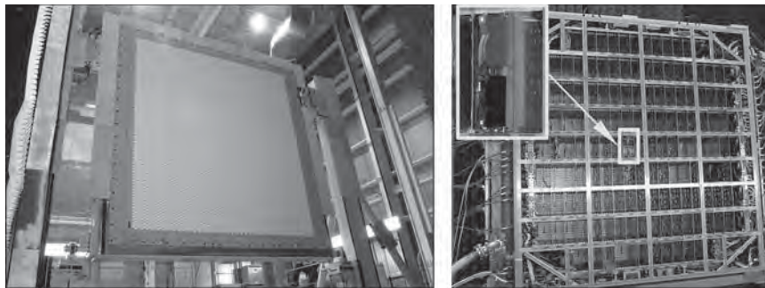
FIGURE 13.43 Front (left) and rear views of Volume Search Radar S-Band engineering development model active phased array mounted in near-field test facility during assembly. Rear view shows detail of easily replaceable lowest replaceable units. (Courtesy of Lockheed Martin Corporation)
