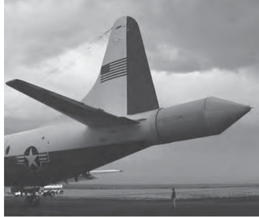
FIGURE 19.12 Tail-mounted ELDORA doppler weather radar operated by the National Center for Atmospheric Research on the Naval Research Laboratory P-3 research aircraft ( Courtesy of University Corporation for Atmospheric Research © 2007, Boulder, CO )
