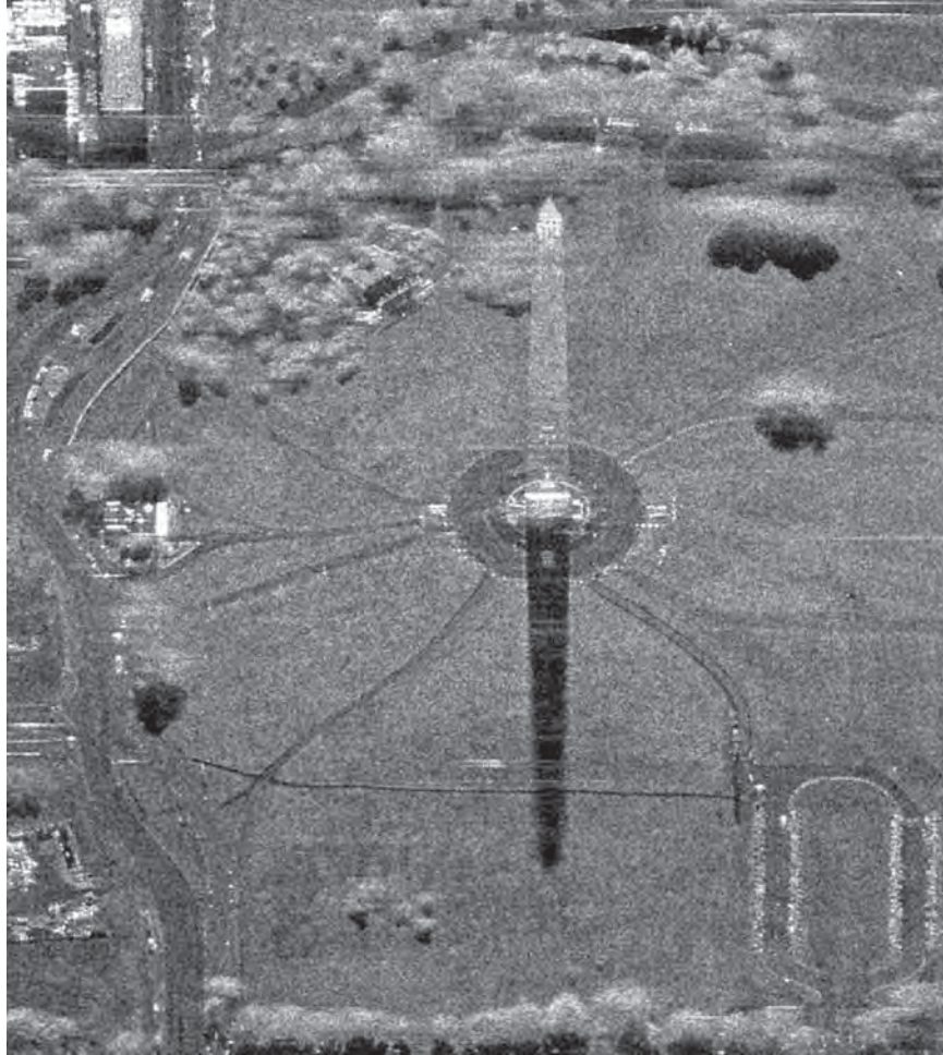
FIGURE 17.9 SAR image of the Washington Monument: The SAR image shows the side of the Monument that is on the opposite side of the shadow, which may appear counterintuitive to a human observer. (Courtesy of General Dynamics, Ypsilanti, Michigan)
