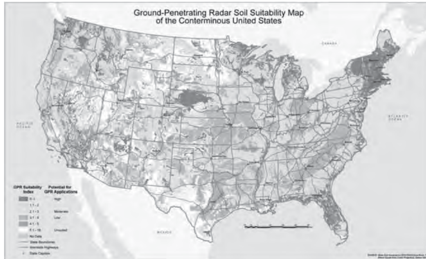
FIGURE 21.15 GPR Soil Suitability Map of the Continental (Conterminous) United States ( Courtesy of USDA-NRCS )
