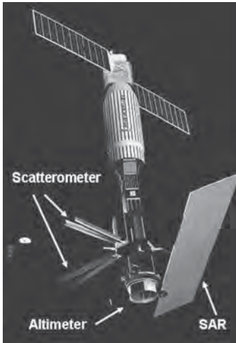
FIGURE 18.1 The Seasat satellite, featuring the antennas of its three radars (Courtesy of NASA)
