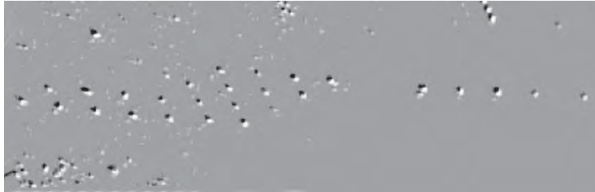
FIGURE 21.36 UWB SAR image of buried AT mines in the Yuma Desert, aircraft at 400 m altitude (Courtesy SRI International USA, Dr. R. Vickers)
