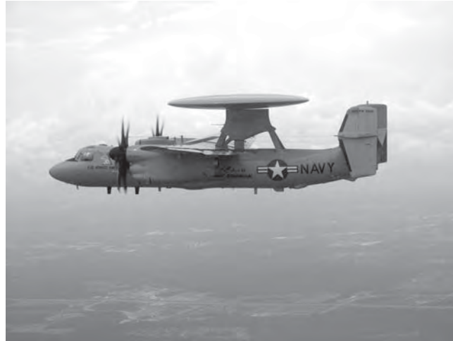
FIGURE 3.1 E-2D airborne early-warning (AEW) aircraft showing rotodome housing the antenna
